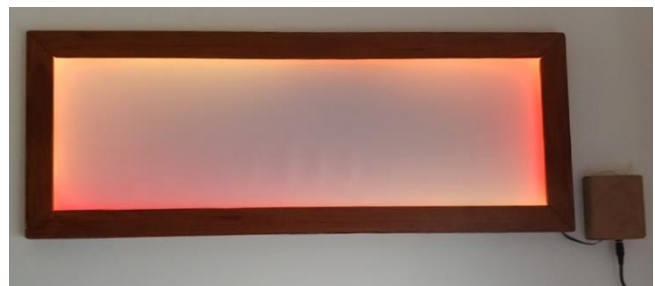
Figure 1. Final research artefact showing the heating status (red) of a smart thermostat
